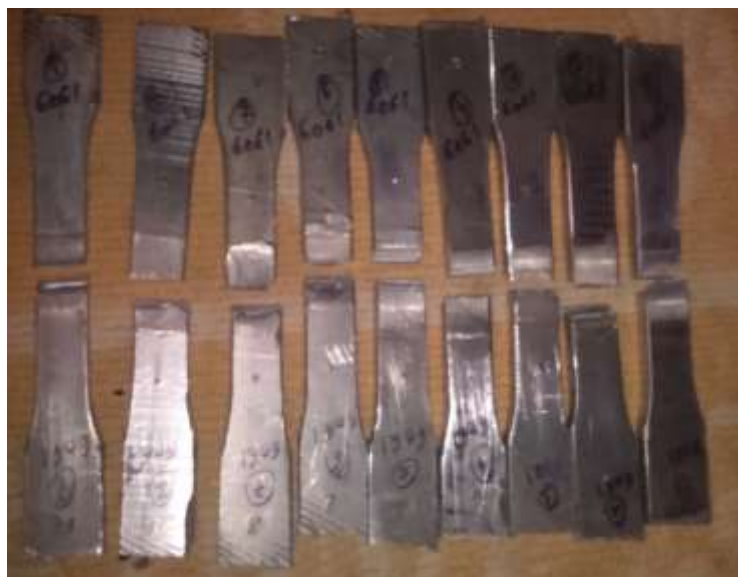
Fig. 3.8 Tensile test specimen after failure
